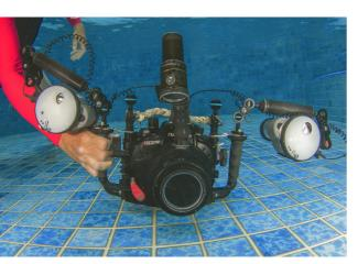
FIG. 6.45 A typical set up for a 60 mm macro position with the strobes just in front of my right hand on the handle. By Sascha Janson.
