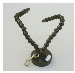
FIG. 8.74 An early version of a dual fibre optic snoot designed to fit on the front of my Inon Z240 strobe and transfer the light along 6 mm fibre optic cables to the subject. The arms are made of flexible hoze-loc and a variety of ends can be fitted to adjust the size of the light beam. This is a useful system if two sources of light are needed.
