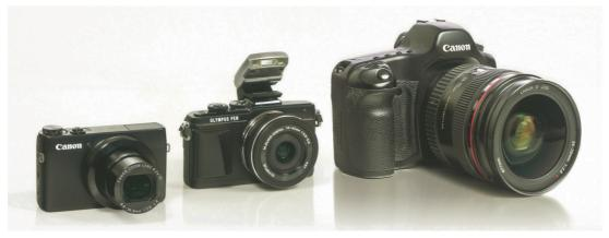
FIG. 2.4 Size comparison. Compact camera on the left, mirrorless in the middle and DSLR on the right.
